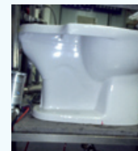
測試器材：排水孔通氣機臺與馬桶底部密封
